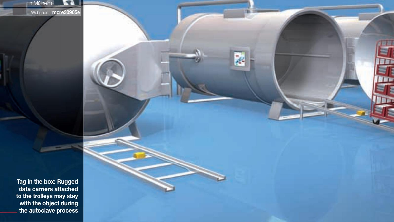
**Tag in the box: Rugged data carriers attached to the trolleys may stay with the object during the autoclave process**
