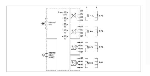
The analog input module Al43-N is used for the connection of potentiometers in 3 or 4wire technology. If 3-wire potentiometers are used, the terminals at the module rack have to be bridged. Resistance measurements, i.e. the evaluation of potentiometers with a 2-wire connection, is not possible.
