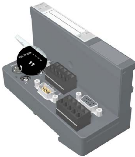
Figure 4-13: DIP-switch to set the transfer rate
