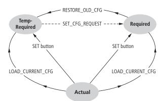
Fig. 17: Accepting the station configuration
