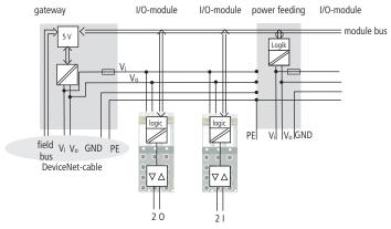
Fig. 40: Block diagram of a BL67 station
