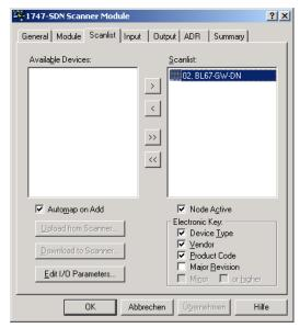
Fig. 30: Incorporating the BL67 Station in the Scan List
