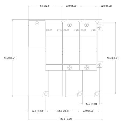
Fig. 4: Dimensions/drilling plan
