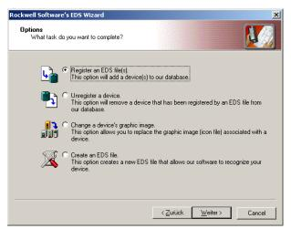
Fig. 23: Registering the EDS File
