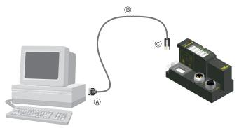
Fig. 9: BL67-gateway connected to PC via special cable
