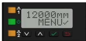
Figure 2. Display shown in Run Mode
