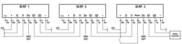
Figure 6. Wiring the switch in series
