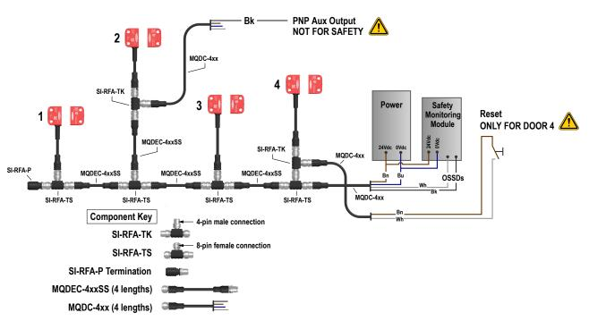
Figure 7. Wiring the switch in series using the quick disconnect connector
