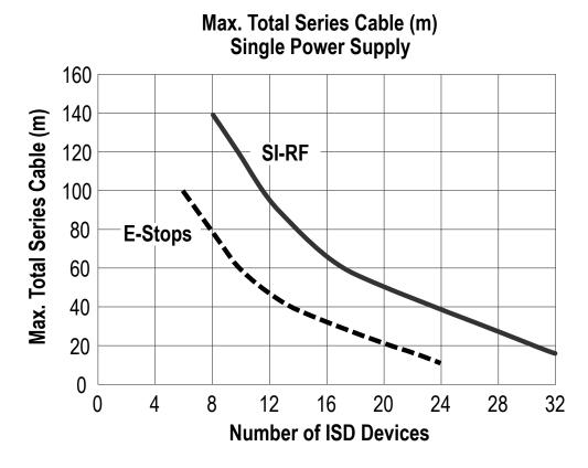
The SI-RFD switches and the ISD Connect have similar current demands. However, when used with a number of lighted ISD emergency stop devices, the current draw of the emergency stop devices governs the cable lengths and when more power is needed.
