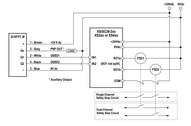
Figure 4. Wiring for a single PNP
