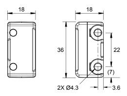
Figure 12. SI-RF Safety Switch Actuator
