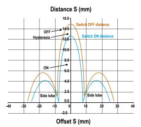
Figure 3. Sensor and actuator active areas
