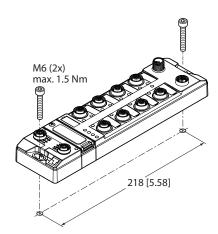
Fig. 5: Mounting the device onto a mounting plate
