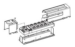
Fig. 4: Installing the device in the TB-SG-L protective housing
