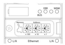
Fig. 11: Rotary coding switches at the device
