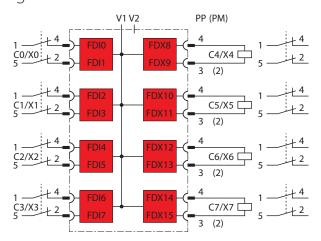
Fig. 3: Block diagram TBEN-LL-4FDI-4FDX
