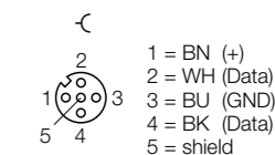
RFID channels (C0...C3) - Connectors .../S2501
